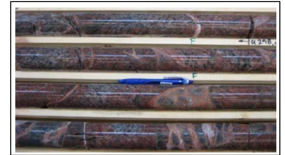
Drill cores with sealed fractures (SKB).
